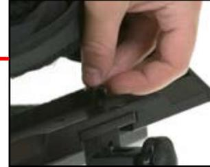
**5** Slide beamsplitter into beamsplitter frame.
